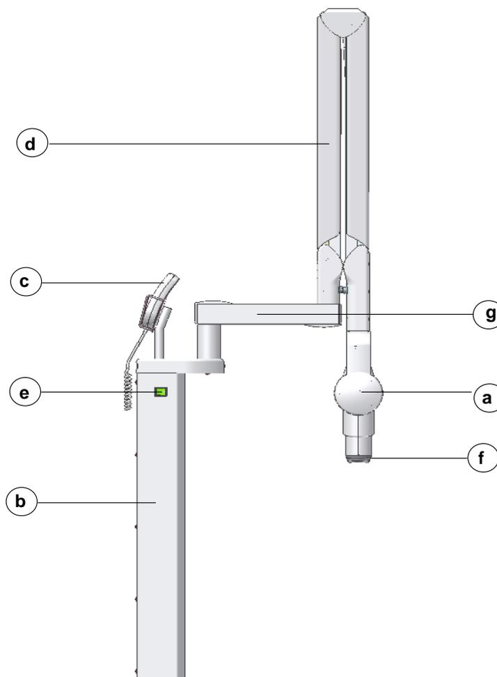
Figure 6. KODAK 2100 Intraoral X-ray System floor-mounted unit
