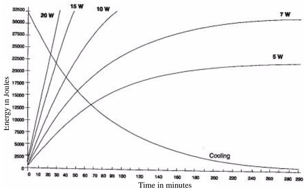
Figure 17. Heating and cooling curves of the KODAK 2100 system tube head
